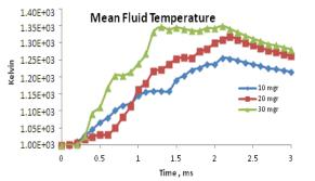
Figure 10. Mean fluid phase temperature versus time for porosity 90 % and different injected fuel
