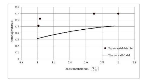
Figure 2. Flame propagation speed as a function of dust concentration for  $50 \sim m$  particles
