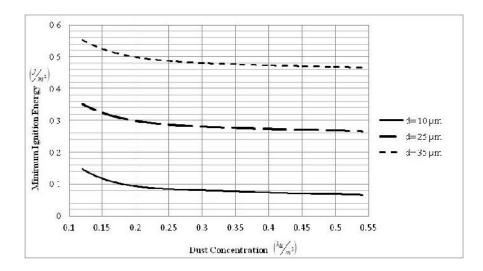
Figure 4. Minimum ignition energy as a function of dust concentration in different particle diameters
