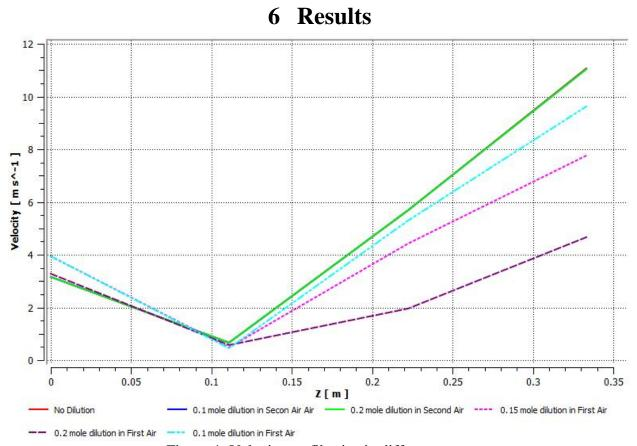
Figure 4- Velocity profiles in six different cases
