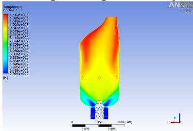
Figure 10- Temperature profile in combustion chamber with 0.15 mole fraction CO<sub>2</sub> in First air zone
