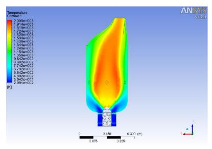
Figure 14- Temperature profile in combustion chamber with 0.2 mole fraction CO<sub>2</sub> in second air zone
