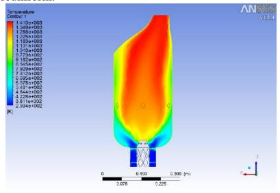
Figure 9- Temperature profile in combustion chamberwith 0.10 mole fraction CO<sub>2</sub> in First air zone
