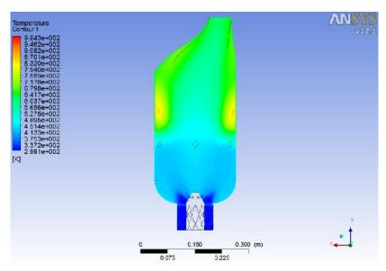
Figure 11- Temperature profile in combustion chamber with 0.2 mole CO<sub>2</sub> dilution in first air zone
