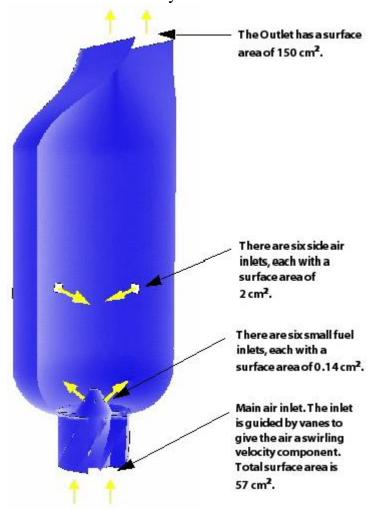
Figure 1- Combustor schematic
