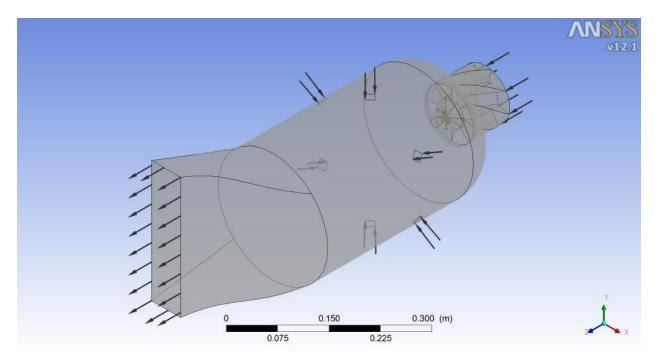
Figure 3- Boundary conditions specified on combustor model
