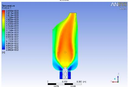
Figure 12- Temperature profile in combustion chamber 0.1 mole fraction of  $CO_2$  in second air zone
