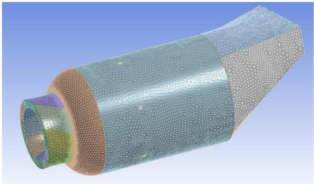
Figure 2- generated grid for combustor model
