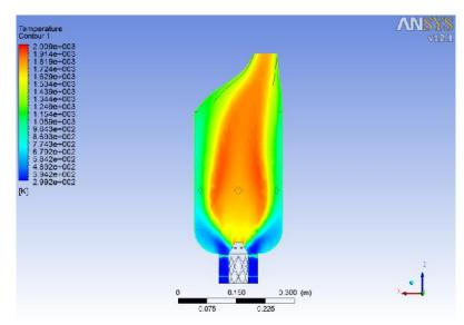
Figure 13- Temperature profile in combustion chamber with 0.15 mole fraction CO<sub>2</sub> in second air zone
