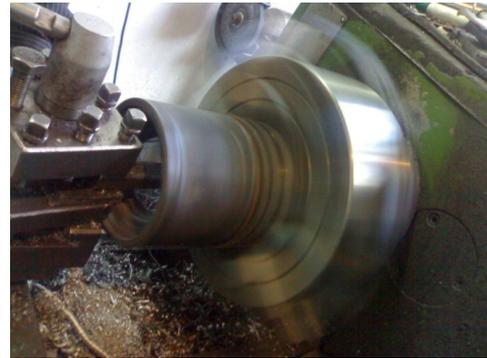
Figure 4. Making a hole from the bottom of the piston
