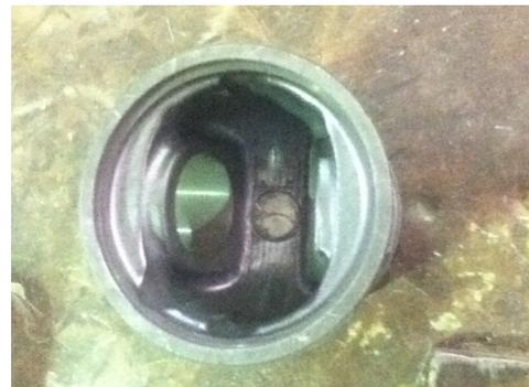
Figure 6. The groove around the bonnet which makes the piston feasible to be welded
