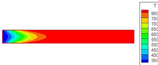
Figure 4. Temperature contours for the base-line conditions
