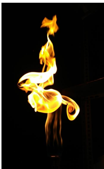
Fuel: Trimethyl Borate - Ozone Mixture Burner: Modified Meker-Fisher Burner
