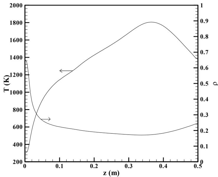
Figure7. Mean temperature and density results along the centerline of the burner.
