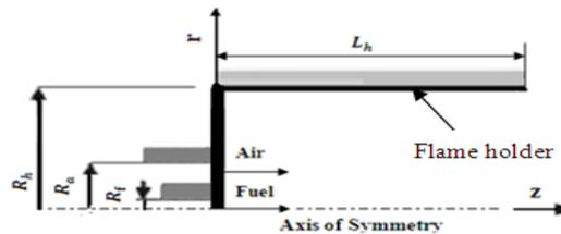
Figure2. Burner configuration.
