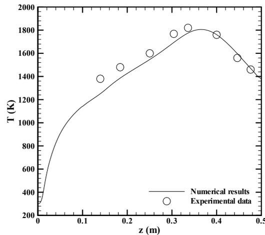
Figure3. Axial distribution of temperature at  $r=0$ : comparison among numerical results and experimental data.
