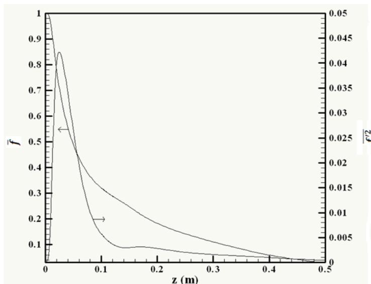
Figure8. Profiles of the mixture fraction and its variance along the axial direction.
