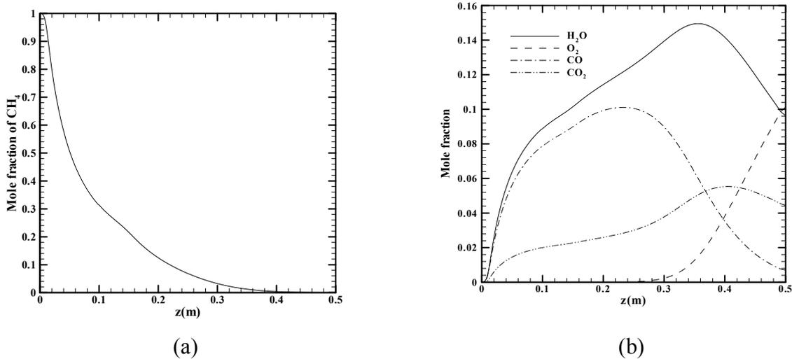
Figure 9. Mean mole fraction of the combustion species at the centerline.
