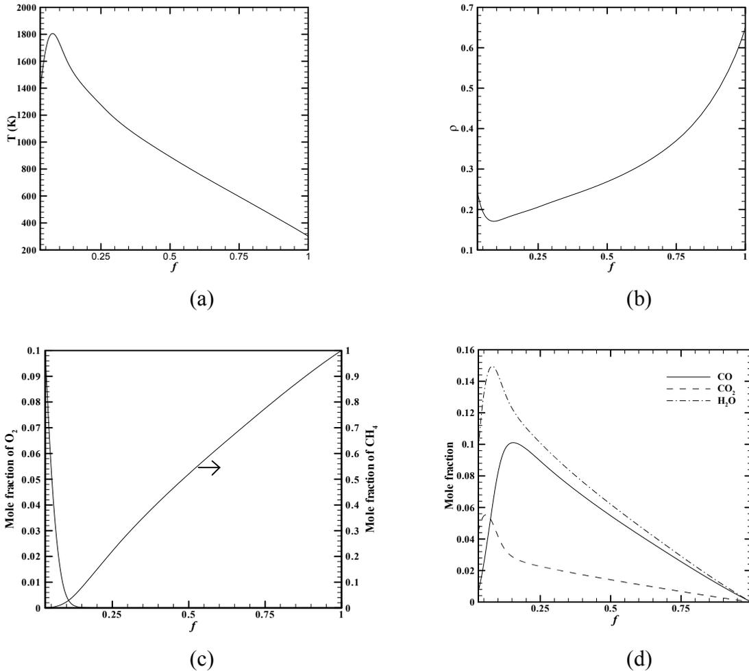
Figure 6. Flame results showing the dependence of the (a) temperature, (b) density and (c)-(d) species mole fractions on the mixture fraction.
