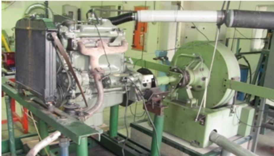
**Figure 1.** The diesel engine experimental set up**Table 1:** Specifications of OM314 diesel engine
