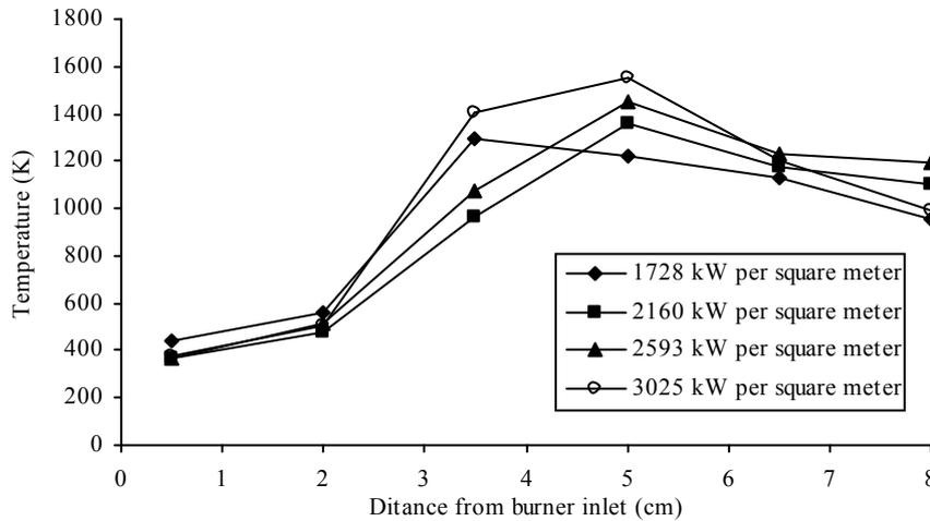
Figure 4. Temperature profiles VS. Burner length at  $\Phi=0.65$
