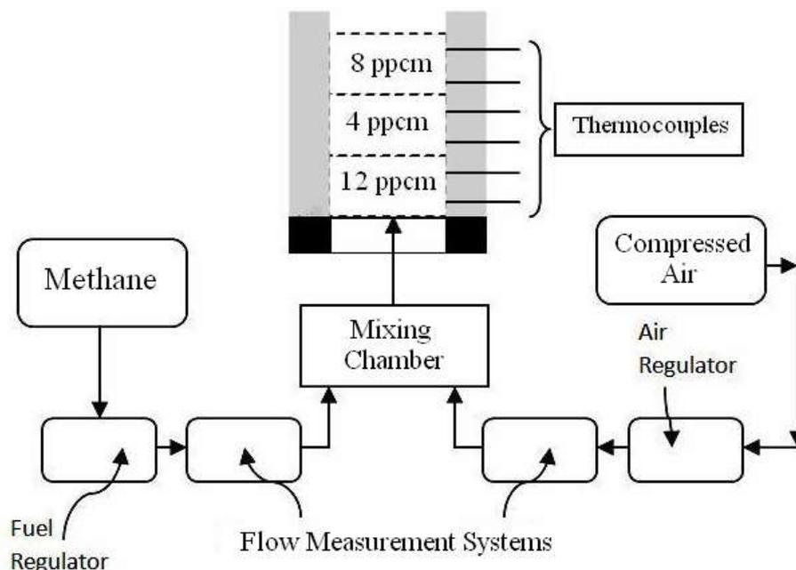
Figure 1. Experimental setup of the present porous burner
