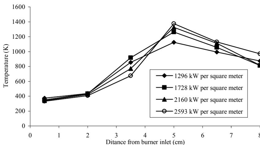
Figure 2. Temperature profiles VS. Burner length at  $\Phi=0.55$
