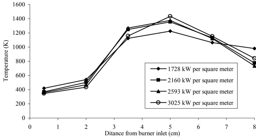
Figure 3. Temperature profiles VS. Burner length at  $\Phi=0.60$
