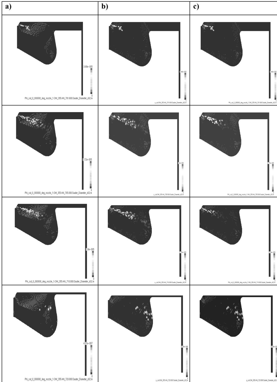
Figure 11 Comparison of SMD in four crank angles (701.6, 705, 710 and 720°C) for different breakup models: a) WAVE b) FIPA c) KH-RT
