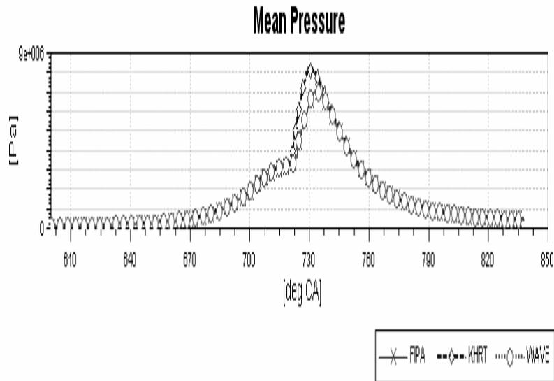
Figure 9 Comparison of cylinder pressure for different Breakup models.
